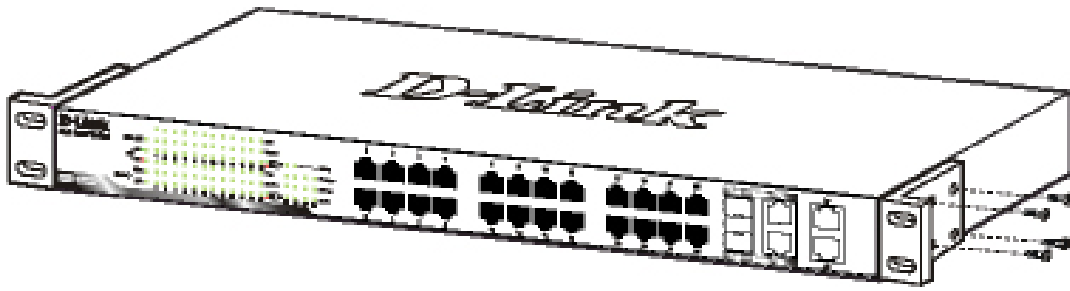
Figure 2 – Attach the mounting brackets to the Switch
