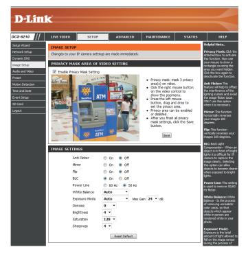
Exposure Mode: Changes the exposure mode. Use the drop-down box to set the camera for Indoor, Outdoor, or Night environments, or to Moving to capture moving objects. The Low Noise option will focus on creating a highquality picture without noise. You can also create 3 different custom exposure modes. The Max Gain setting will allow you to control the maximum amount of gain to apply to brighten the picture.
