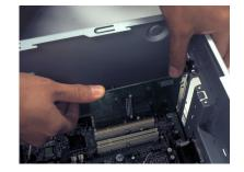
After the PCI Card Holder is secured, then insert the PCI Card, facing down as shown, into the PCI Card Holder.
