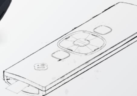
Pull out the plastic tab from the remote to activate the battery.
