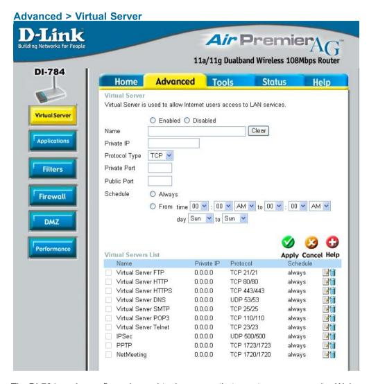
The DI-784 can be configured as a virtual server so that remote users accessing Web or FTP services via the public IP Address can be automatically redirected to local servers in the LAN (Local Area Network).
