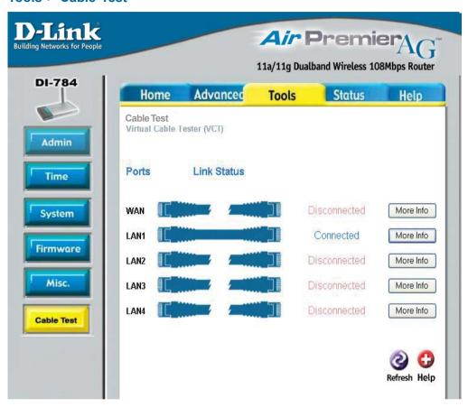
**Cable Test** is an advanced feature that integrates a LAN cable tester on every Ethernet port on the router. Through the graphical user interface (GUI), **Cable Test** can be used to remotely diagnose and report cable faults such as opens, shorts, swaps, and impedance mismatch. This feature significantly reduces service calls and returns by allowing users to easily troubleshoot their cable connections.
