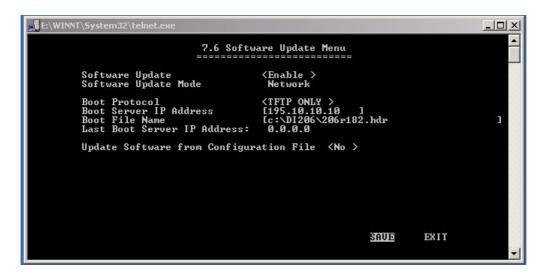
Setup as above saving the settings. Now Reboot the router, either by powering down router or selecting - Main Menu – System Maintenance – System Restart.
