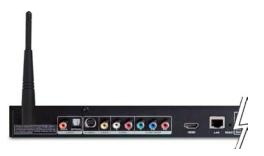
**Note:** You may have an Ethernet cable plugged into the unit and have the wireless antenna connected. Neither will interfere with the other, but only one network can be accessed at a time (wired or wireless). The network connection type is selected in the Setup Wizard and can be changed by going to the Setup Menu. To access the Setup Menu, press the SETUP button on the remote control.
