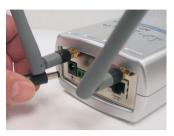
When you have a proper connection, the LED (Light Emitting Diode) on the front of the camera will turn from red to green. The light may blink on and off and your computer may show an intermittant loss of connectivity, this is normal until you have configured your camera.
