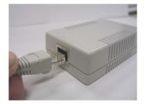
Insert one end of the DC 5V Power Cable that is provided into the Terminal Unit, and the other end into the DC 5V of the Wireless Access Point. The green LED of the Terminal Unit should light up.
