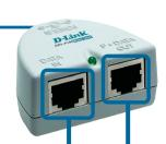
**Data In**: connect an RJ-45 straight-through cable to your computer or switch.
