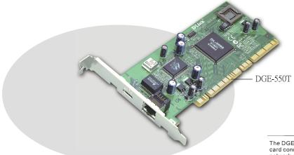
The DGE-550T Gigabit PCI card for server connection. This card connects to the Cat. 5 twisted-pair cable, common at most network sites, to transfer data at a blazing 2000Mbps full duplex speed, eliminating all networkbottlenecks.
