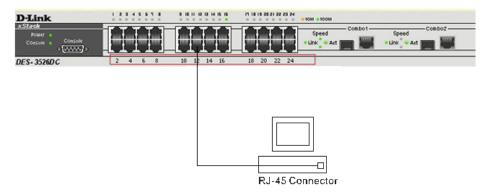
Figure 3-1. DES-3526 connected to an end node
