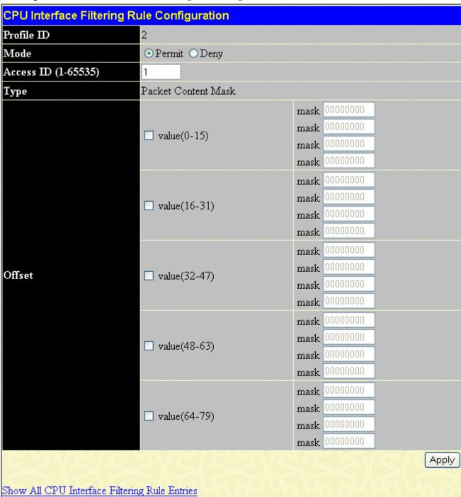
Figure 6- 97. CPU Interface Filtering Rule Configuration window for Packet Content Mask
