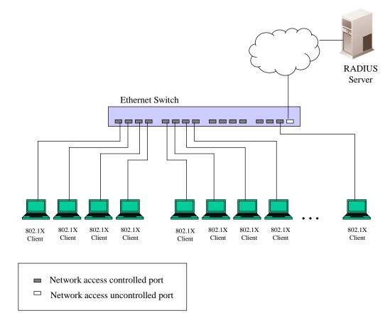
Figure 7- 10. Example of Typical Port-Based Configuration
