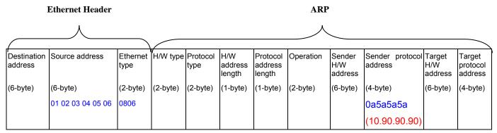
Table-7: A completed ARP packet contained in Ethernet frame
