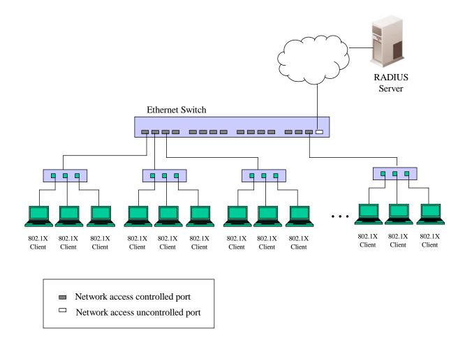
Figure 7- 11. Example of Typical MAC-Based Configuration
