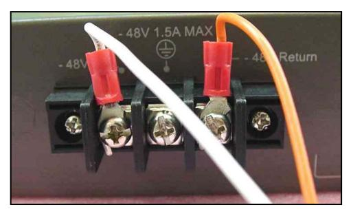
Figure 2-7. Power connections attached to contacts on assembly
