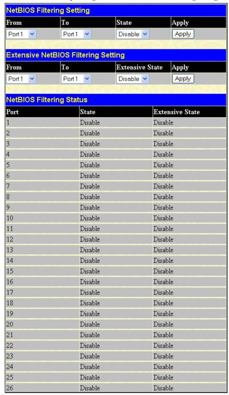
Figure 7- 62. NetBIOS Filtering Setting and Extensive NetBIOS Filter Setting window
