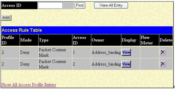
Figure 6- 104 Access Rule Table for IP-MAC Binding rule (Modify)
