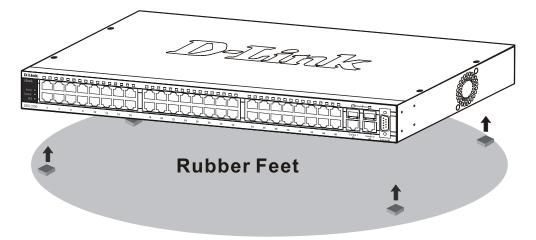
Figure 2- 2. Preparing the DES-3550 for installation on a desktop or shelf
