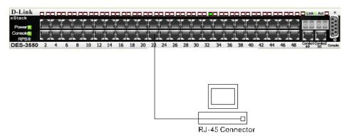
Figure 3- 2 DES-3550 connected to an end node
