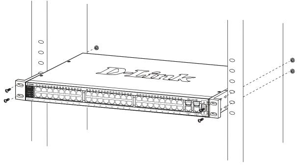
Figure 2- 6. Installing the DES-3550 in a rack
