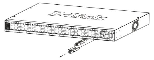
Figure 1- 12. Inserting the Mini-GBIC modules into the DES-3550
