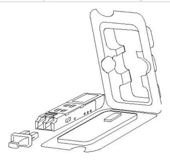
Figure 1-13. Installing the Mini-GBIC Module
