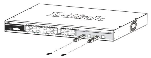
Figure 1- 11. Inserting the Mini-GBIC modules into the DES-3526
