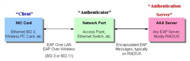
Figure 7-6. Three Functions of 802.1x
