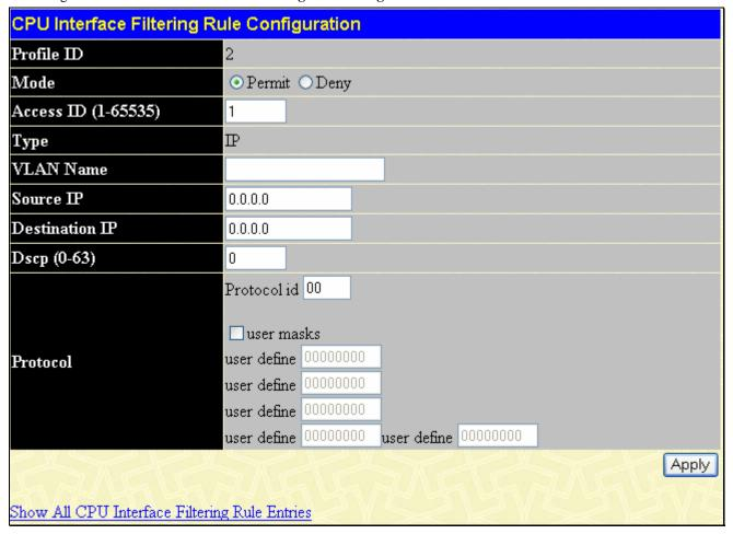
Figure 6-95. CPU Interface Filtering Rule Configuration window for IP
