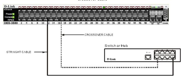
Figure 3- 4 DES-3550 connected to a normal (non-Uplink) port on a hub or switch using a straight or crossover cable
