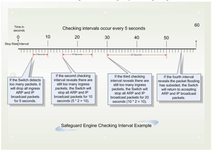
Figure 7-57. Safeguard Engine example
