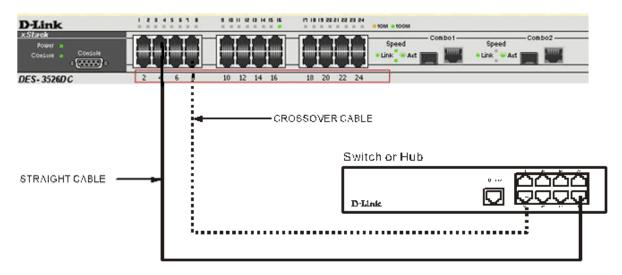
Figure 3- 3. DES-3526 connected to a normal (non-Uplink) port on a hub or switch using a straight or crossover cable
