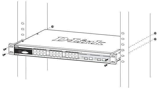
Figure 2-5. Installing the DES-3526 in a rack
