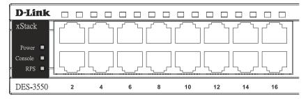
Figure 1-5. Indicators on DES-3550 Series switch
