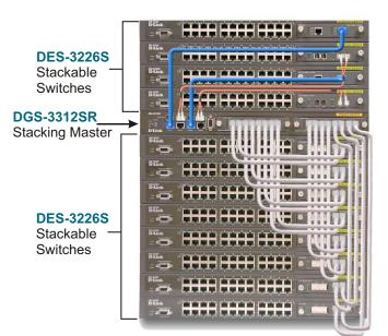
Stack of 12 DES-3226S switches connected to a DGS-3312SR Stacking Master in a star stacking scheme. 8 DES-3226S are connected to the Stacking Master through their stacking ports. 4 other DES-3226S are stacked with stacking Master through the Gigabit ports.
