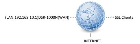
Here we are trying to build a SSL VPN server on the DSR-1000N for users who are able to remotely connect into the resource of a company network.
