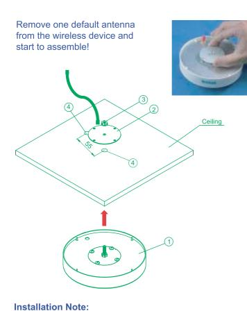
1. Carefully remove the antenna from the package. 2. Take out the Washer (1 pcs) from the package 3. Take out the Flange washer (1 pcs) as well. 4. Drill 2 holes through the ceiling board, one to fix the antenna main body with wacher, another for the antenna SMA connector linked onto extension
