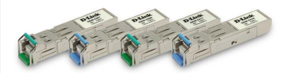
The DEM-330T/330R and DEM-331T/331R Bidirectional Gigabit SFP Fiber Transceivers are external transceivers designed for insertion in SFP (Small Form-Factor Pluggable) slots of network devices for transmission and reception of data signals on the fiber cables. These transceivers provide the Gigabit operation and physical compactness to deliver the speed, reliable long-distance data transfer, and deployment flexibility that today's fiber networks require.
