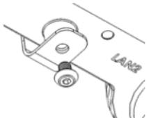
Use the included mount screw (hexagonal hole) to lock the DAP-3662 to the pole/wall mount
