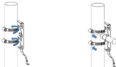
Secure mount base to the pole with two stainless tie back strap sets. Ensure that the tie back is locked securely.
