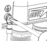
Tighten the grounding wire to the DAP-3662 until it is securely attached.
