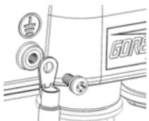
Attach the grounding wire to the DAP-3662 using the included screw.
