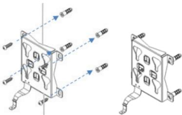
Securely mount the base to the wall using wall plug and wall screw.
