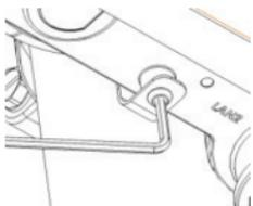
With the included hexagon socket spanner, tighten the mount screw until the DAP-3662 is secured.
