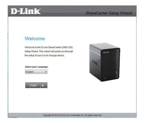
**Note:** The computer used to access the ShareCenter Pulse web-based configuration manager must be on the same subnet as the ShareCenter Pulse. If your network is using a DHCP server, the ShareCenter Pulse will automatically be in the same subnet.
