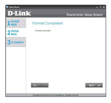
The final window of the installation wizard shows successful completion. Your device is now installed and ready for use. Your drives are network mapped from using the wizard so you will be able to access them under you *My Computer* icon.
