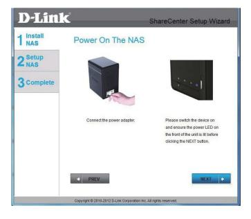
With the power on check that the Power LED is solid. If it is solid, answer **Yes** to the confirmation window otherwise select **No** and wait for the power connection to the ShareCenter Pulse. If the connection is good then check that the hard drives are installed correctly and have no other issues. Click **Next** to continue.
