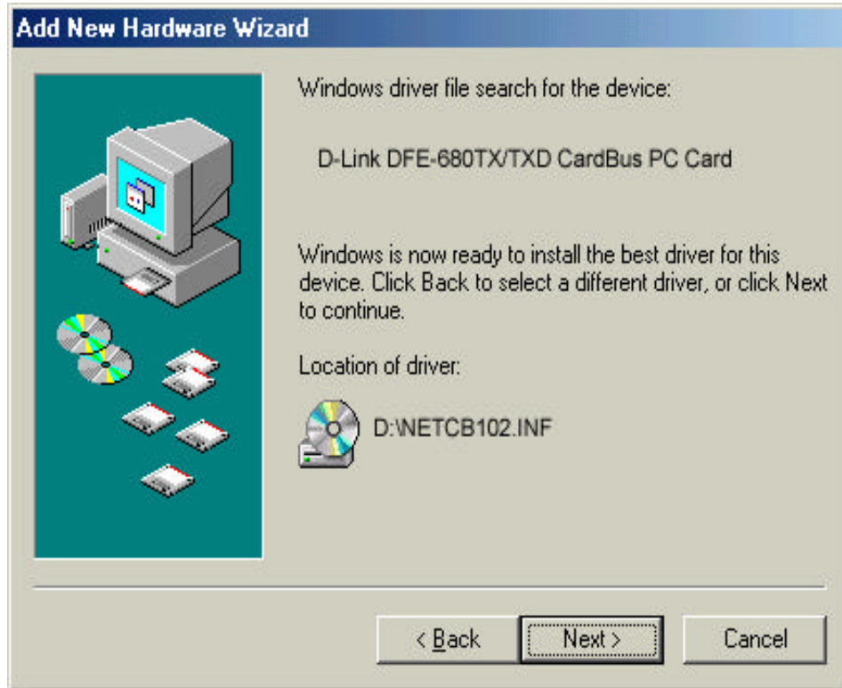
Figure3- A screen appears telling you that is has located the DFE-680TXD driver in the CD-ROM drive. Then click Next , Windows will copy files to the hard drive.
