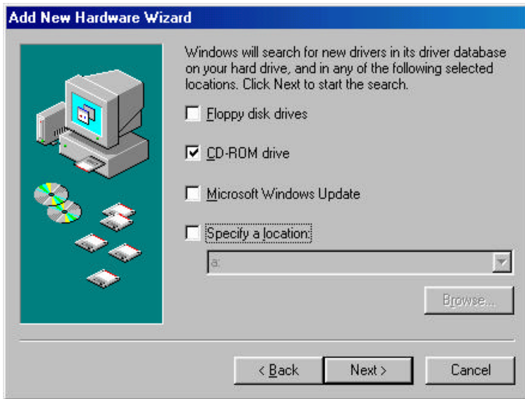
Figure3- Enter CD-ROM drive, or click on the Browse button and select CD-ROM drive.
