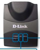
indicates that the wireless segment is ready. This LED blinks during wireless data transmission.
