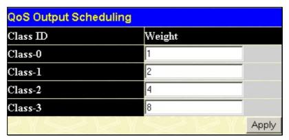
Figure 8-6. QoS Output Scheduling Configuration window
