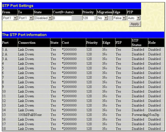
Figure 7-15. STP Port Settings and Table window
