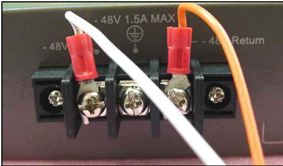
Figure 2- 5. Power connections attached to contacts on assembly
