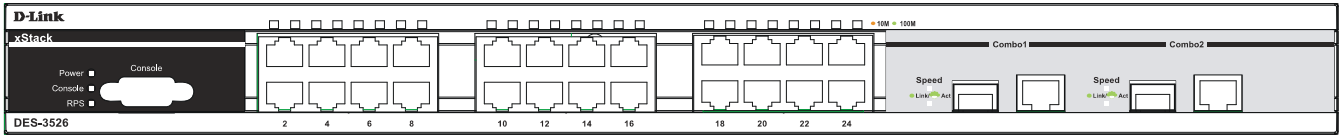
Figure 1- 1. Front Panel View of the DES-3526 switch
