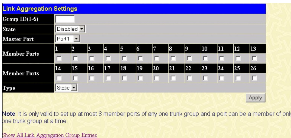
Figure 6- 9. Link Aggregation Settings window – Add
