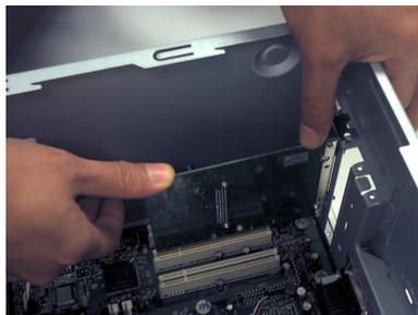
After the PCI Card Holder is secured, then insert the PCI Card, facing down as shown, into the PCI Card Holder. Press the PC Card firmly into the PCI holder.
