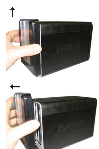
3. Insert a 3.5" SATA hard drive into each available drive bay. Make sure to align the drive connectors to the endpoints in the DNS-323. Gently push the drive in until it connects.
