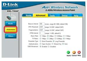
remain at its default setting of 2,347. If you experience a high packet error rate, you may slightly increase your fragmentation threshold within the value range of 256 to 2,346. Setting the fragmentation threshold too low may result in poor performance.
