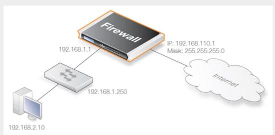
A D-Link switch model DES-3226S is used in this case, with a management interface address 192.168.1.250 connecting to the firewall's interface address 192.168.1.1. This firewall interface is added into the exclude list to prevent the firewall from being accidentally locked out from accessing the switch.
