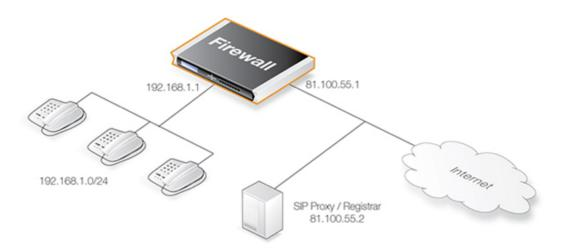
The SIP proxy in the above diagram could alternatively be located remotely across the Internet. The proxy should be configured with the **Record-Route** feature enabled to insure all SIP traffic to and from the office clients will be sent through the SIP Proxy. This is recommended since the attack surface is minimized by allowing only SIP signalling from the SIP Proxy to enter the local network.
