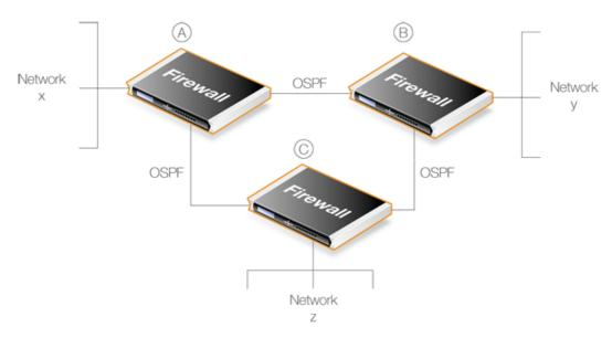
Figure 4.9. OSPF Providing Route Redundancy
