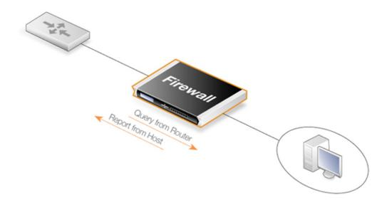
Figure 4.16. Multicast Snoop Mode
