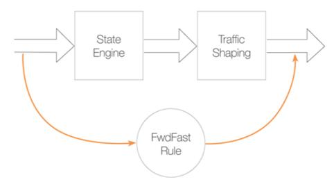
Figure 10.2. FwdFast Rules Bypass Traffic Shaping
