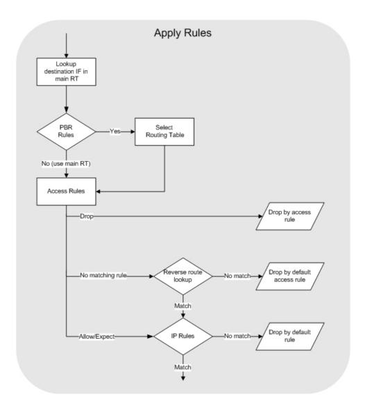
Figure 1.4. Expanded Apply Rules Logic
