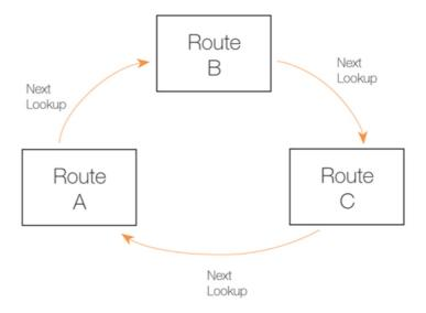
Figure 4.5. The RLB Round Robin Algorithm
