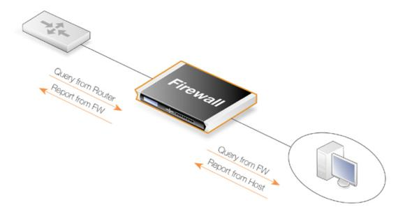
Figure 4.17. Multicast Proxy Mode
