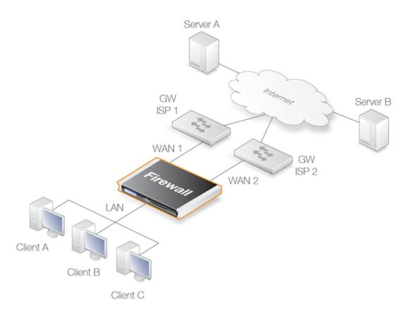
Figure 4.7. A Route Load Balancing Scenario
