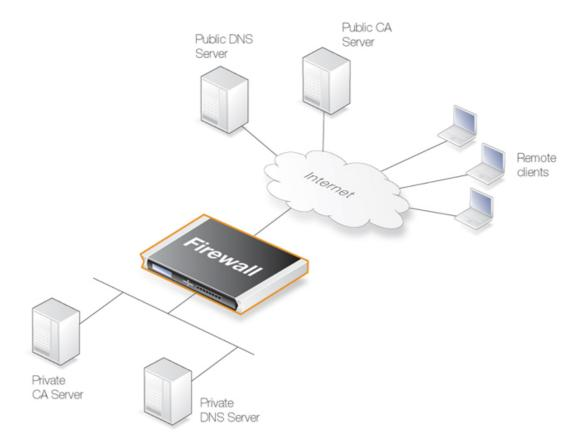
Figure 9.4. Certificate Validation Components
