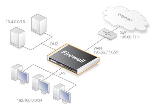
Figure 4.1. A Typical Routing Scenario
