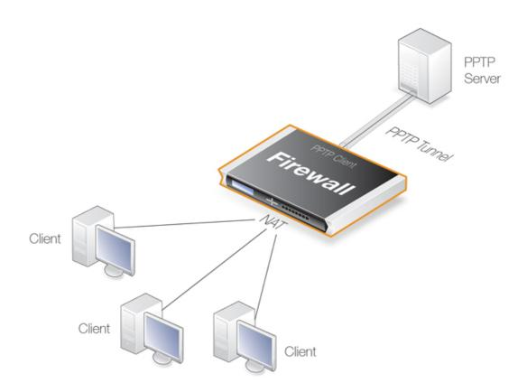
Figure 9.3. PPTP Client Usage
