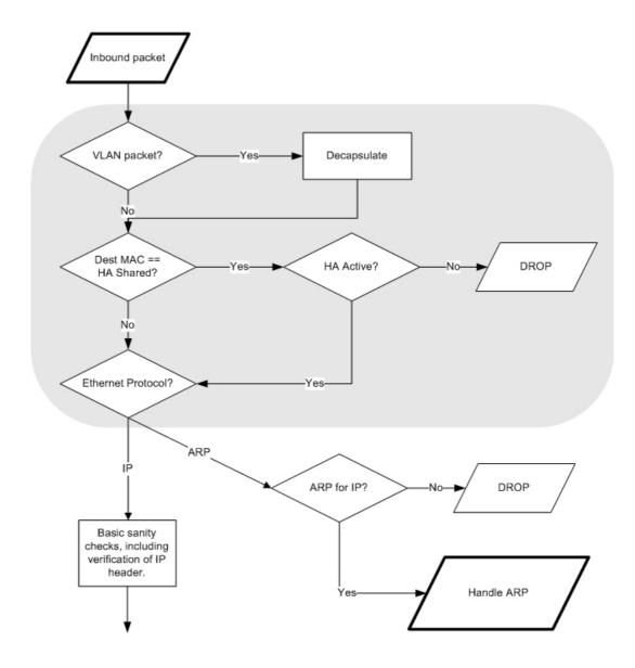
Figure 1.1. Packet Flow Schematic Part I
