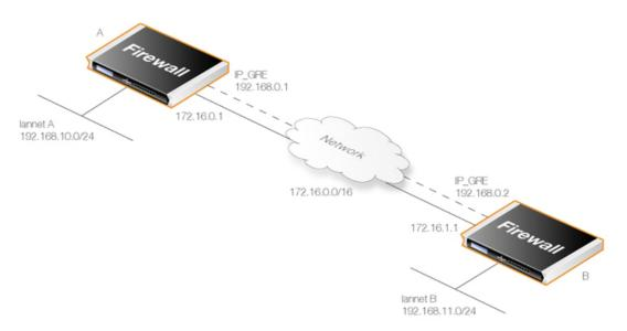
The diagram above shows a typical GRE scenario, where two NetDefend Firewalls **A** and **B** must communicate with each other through the intervening internal network 172.16.0.0/16.
