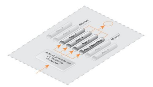
Figure 10.5. Minimum and Maximum Pipe Precedence
