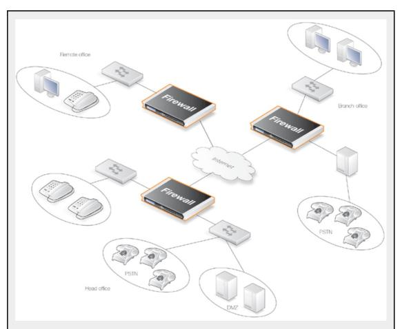
The head office has placed a H.323 Gatekeeper in the DMZ of the corporate NetDefend Firewall. This firewall should be configured as follows:
