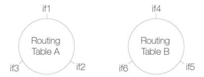
The diagram above illustrates how switch route interconnections for one routing table are completely separate from the switch route interconnections for another routing table. By using different routing tables in this way we can create two separate transparent mode networks.
