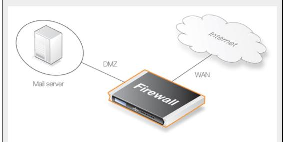
An IDP rule called *IDPMailSrvRule* will be created, and the *Service* to use is the SMTP service. Source Interface and Source Network defines where traffic is coming from, in this example the external network. The *Destination Interface* and *Destination Network* define where traffic is directed to, in this case the mail server. *Destination Network* should therefore be set to the object defining the mail server.
