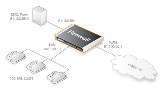
The complexity is increased in this scenario since SIP messages flow across three interfaces: the receiving interface from the call initiator, the DMZ interface towards the proxy and the destination interface towards the call terminator. This the initial messages exchanges that take place when a call is setup in this scenario are illustrated below:
