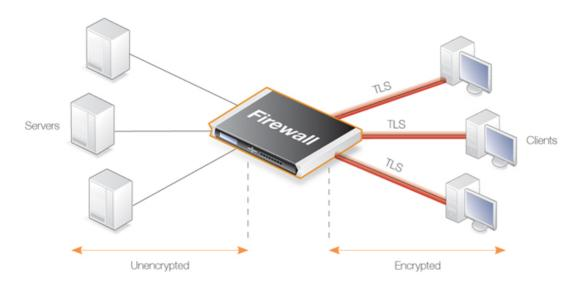
Figure 6.7. TLS Termination
