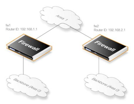
Figure 4.11. Virtual Links with Partitioned Backbone
