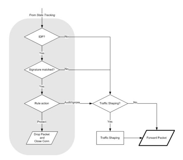
Figure 1.3. Packet Flow Schematic Part III
