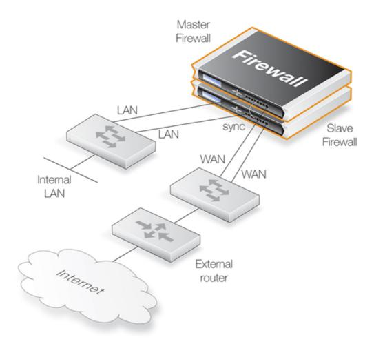
In the scenario shown above, the **lan** interface on the master and the **lan** interface on the slave would be connected to the same switch which then connects to an internal network. Similarly the **wan** interface on the master and the **wan** interface would connect to a switch which in turn connects to the external Internet.
