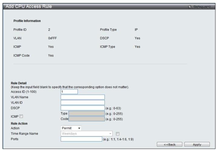
Figure 7-32 Add CPU Access Rule (IPv4 ACL)
