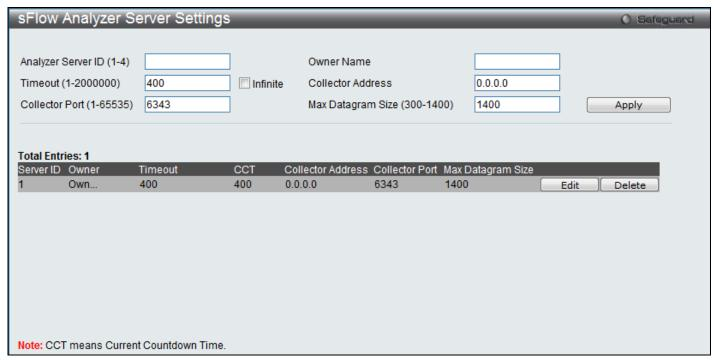
Figure 11-20 sFlow Analyzer Server Settings window
