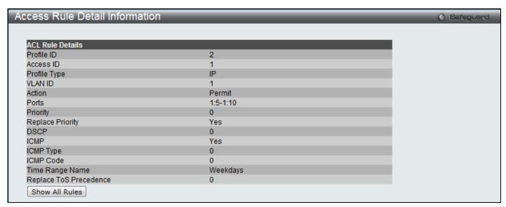
Figure 7-12 Access Rule Detail Information (IPv4 ACL)
