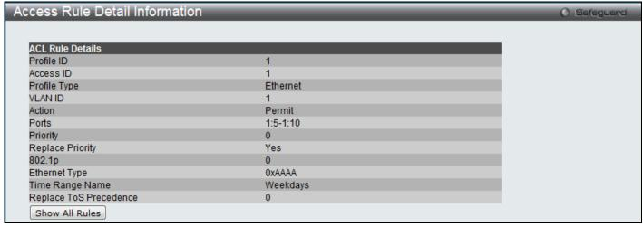
Figure 7-7 Access Rule Detail Information window (Ethernet ACL)
