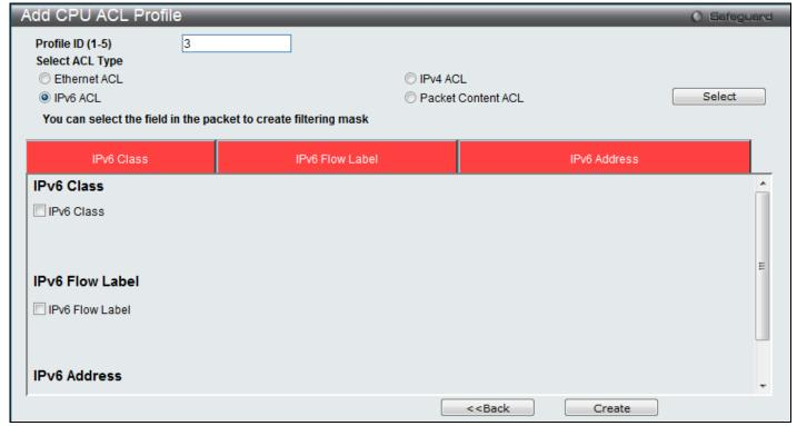
Figure 7-34 Add CPU ACL Profile (IPv6 ACL)
