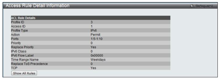
Figure 7-17 Access Rule Detail Information (IPv6 ACL)
