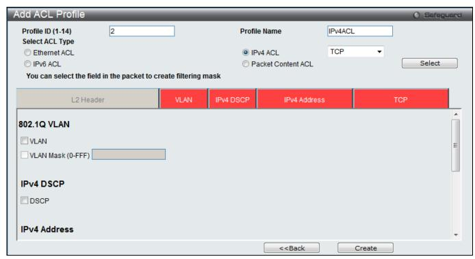
Figure 7-8 Add ACL Profile window (IPv4 ACL)
