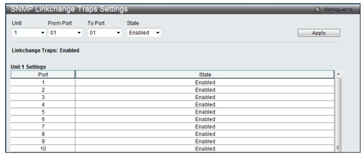
Figure 3-35 SNMP Linkchange Traps Settings window
