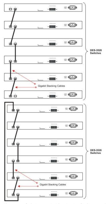
Figure 2-26 Switches stacked in a Duplex Chain
