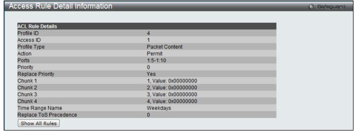
Figure 7-22 Access Rule Detail Information (Packet Content ACL)
