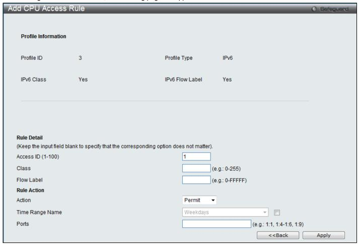
Figure 7-37 Add CPU Access Rule (IPv6 ACL)
