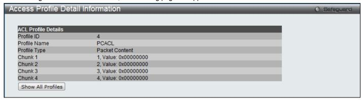
Figure 7-19 Access Profile Detail Information (Packet Content ACL)
