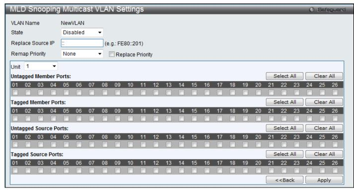
Figure 4-73 MLD Snooping Multicast VLAN Settings – Edit window
