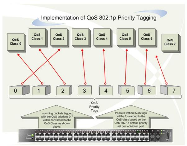
Figure 6-1 Mapping QoS on the Switch
