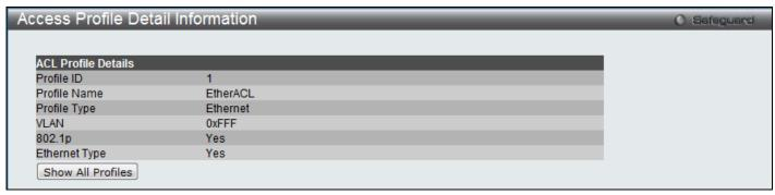
Figure 7-4 Access Profile Detail Information window (Ethernet ACL)
