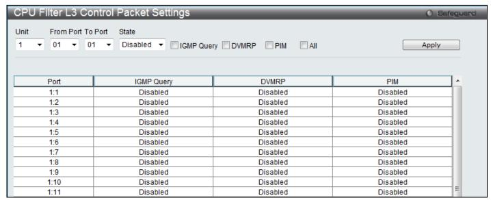
Figure 3 - 2 CPU Filter L3 Control Packet Settings window
