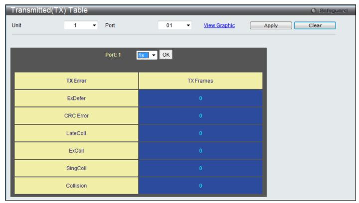
Figure 11-13 Transmitted (TX) Table window (for errors)
