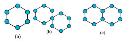
Figure 4-80 Ethernet ring topologies supported by ERPS
