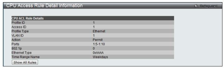
Figure 7-28 CPU Access Rule Detail Information (Ethernet ACL)
