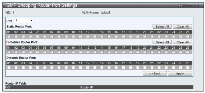
Figure 4-44 IGMP Snooping Router Port Settings window
