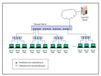
Figure 8-8 Example of Typical Host-based Configuration
