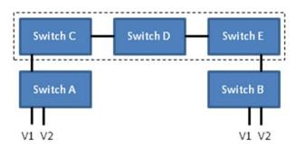
Figure 4-22 Example of VLAN Trunk
