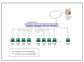
Figure 8-7 Example of Typical Port-based Configuration
