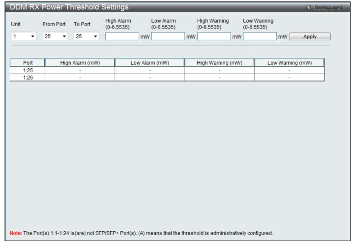
Figure 2-8 DDM RX Power Threshold Settings window
