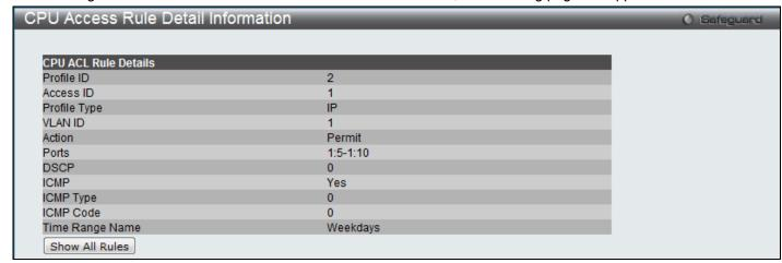
Figure 7-33 CPU Access Rule Detail Information (IPv4 ACL)
