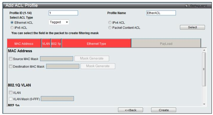
Figure 7-3 Add ACL Profile window (Ethernet ACL)
