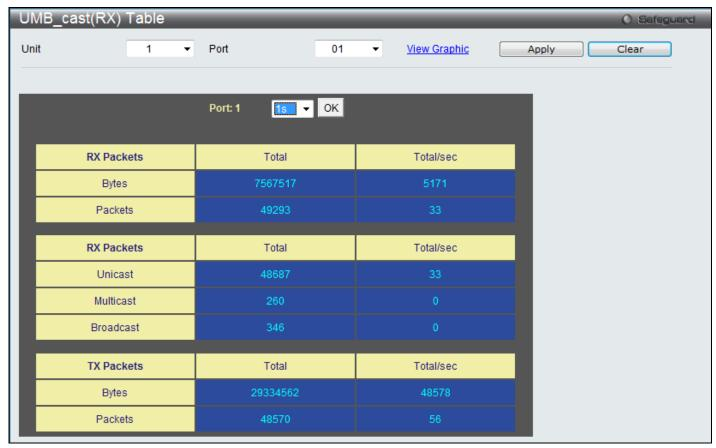
Figure 11-7 RX UMB\_cast (RX) Table window (table for Unicast, Multicast, and Broadcast Packets)
