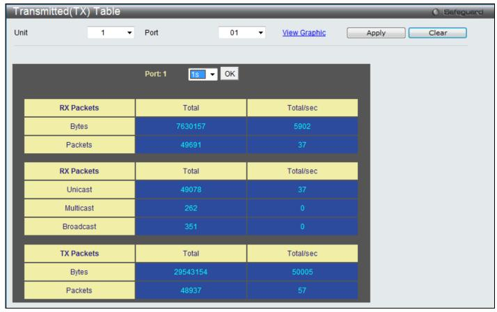
Figure 11-9 Transmitted (TX) Table window (table for Bytes and Packets)
