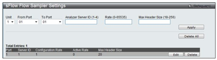
Figure 11-21 sFlow Flow Sampler Settings window
