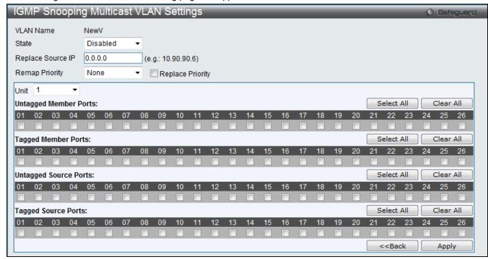
Figure 4-68 IGMP Snooping Multicast VLAN Settings – Edit window
