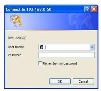
Enter the appropriate User name and Password into the fields above and click the OK button. Your PC's web browser will open and the Access Point's IP address will be entered into the address field. You can then configure the Access Point using its built-in web-based manager as you would normally. There is no difference in using an Access Point's web-based manager initiated by the AP Manager II or any other method.
