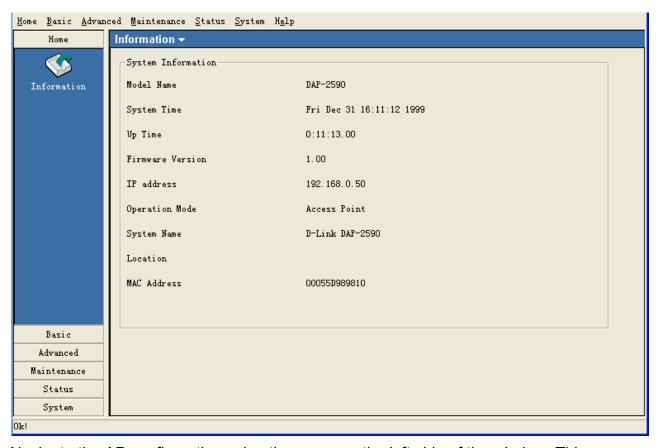
Navigate the AP configuration using the menu on the left side of the window. This menu contains the following sections, **Home, Basic, Advanced, Maintenance, Status,** and **System**. These sections and their menus will be discussed in detail in the following pages.
