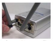
When you have a proper connection, the LED will turn from **red** to **green**. The light may cycle on and off and your computer may show an intermittent loss of connectivity, this is normal until you have configured your Internet Camera.
