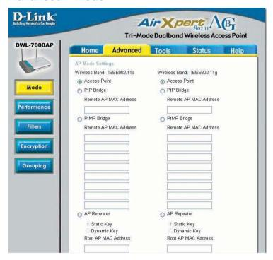
PtMP Bridge (Point to Multi-Point Bridge): This mode enables you to connect multiple WLANs
