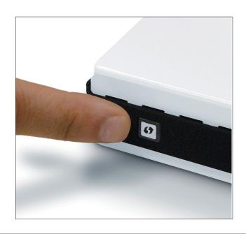
Press the WPS button on the adapter and holding for two seconds until the utility screen comes up. Then, press the WPS button on the router/access point to continue.
