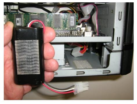
Figure A-4 Aligning the Battery
