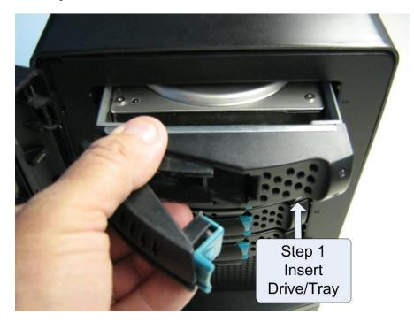
Figure A-21 Drive/Tray Installation
