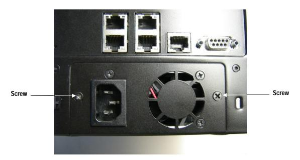
Figure A-24 Remove These Two Screws on the Rear of the Chassis
