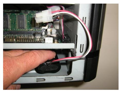
2. Press the battery down firmly as shown in Figure A-5 until you feel it lock into place.
