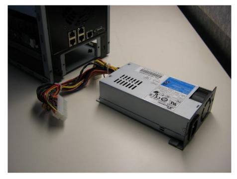
Figure A-28 Remove the Power Supply Harness Connector
