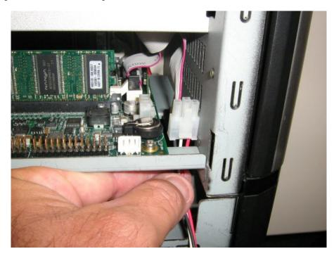
Figure A-6 Align the Battery Plug with Connector J11
