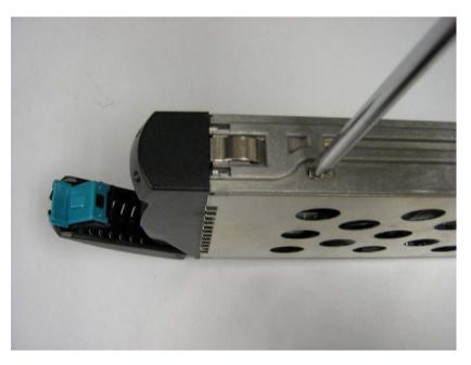
Figure A-20 Secure the Hard Drive in the Drive Tray
