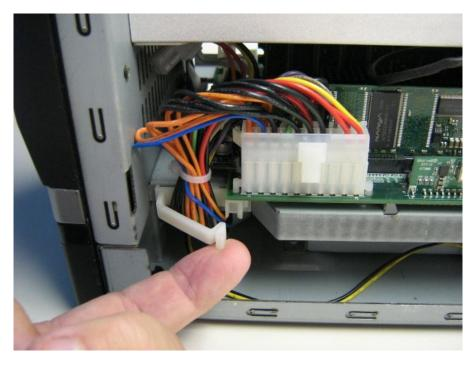
Figure A-26 Open the Power Supply Harness Retention Clip
