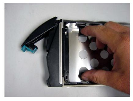
Figure A-17 Removing the Plastic Air Dam Piece
