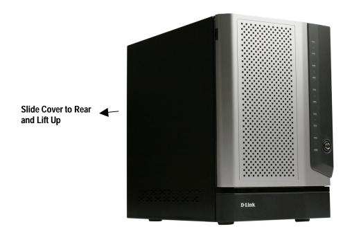
Figure A-2. Slide the Cover Back and Remove
