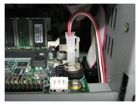
Figure A-8 Battery Plug Locked in Place
