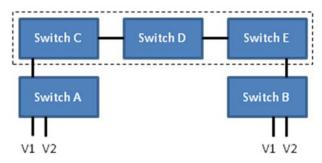
Figure 4-22 Example of VLAN Trunk
