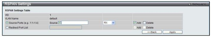
Figure 11-18 RSPAN Settings – Modify window
