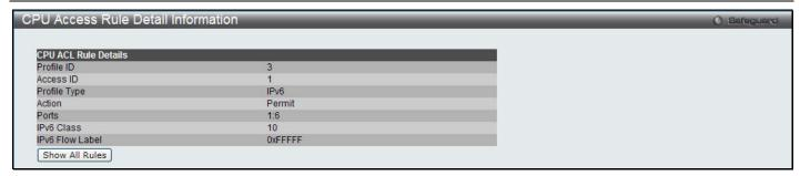
Figure 7-38 CPU Access Rule Detail Information (IPv6 ACL)
