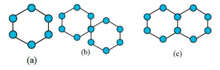
Figure 4-80 Ethernet ring topologies supported by ERPS
