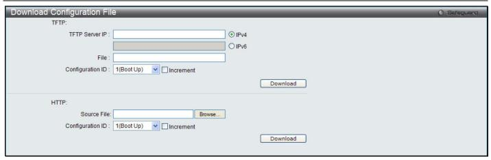
Figure 12-7 Download Configuration – TFTP window
