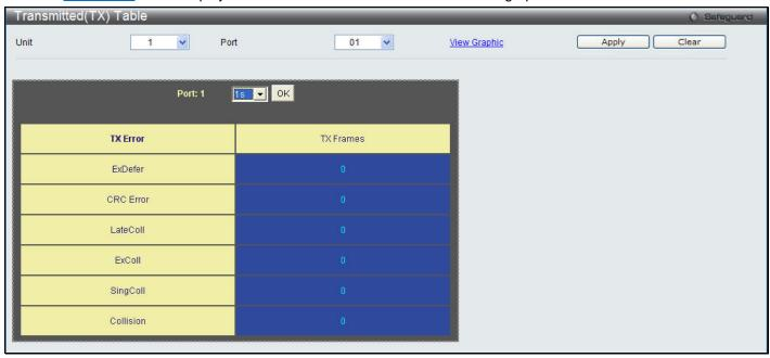
Figure 11-13 Transmitted (TX) Table window (for errors)
