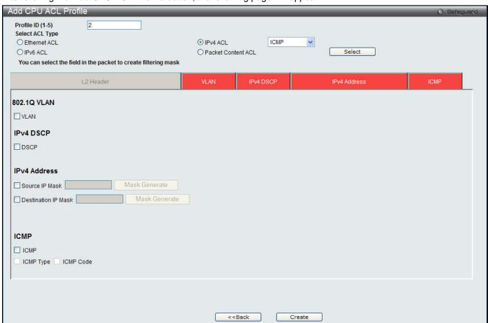
Figure 7-29 Add CPU ACL Profile (IPv4 ACL)
