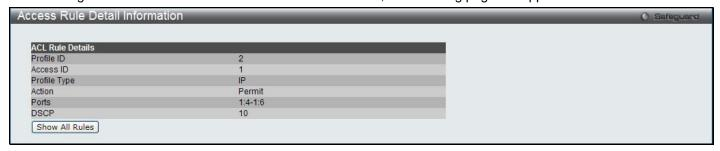
Figure 7-12 Access Rule Detail Information (IPv4 ACL)
