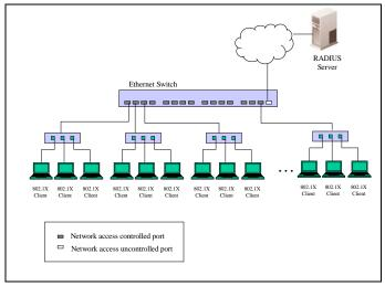
Figure 8-8 Example of Typical Host-based Configuration
