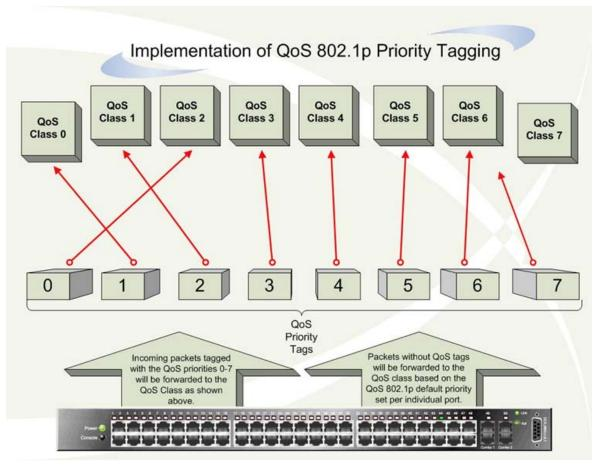
Figure 6-1 Mapping QoS on the Switch
