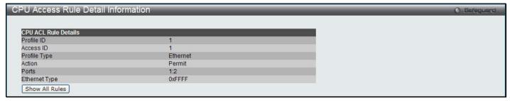
Figure 7-28 CPU Access Rule Detail Information (Ethernet ACL)
