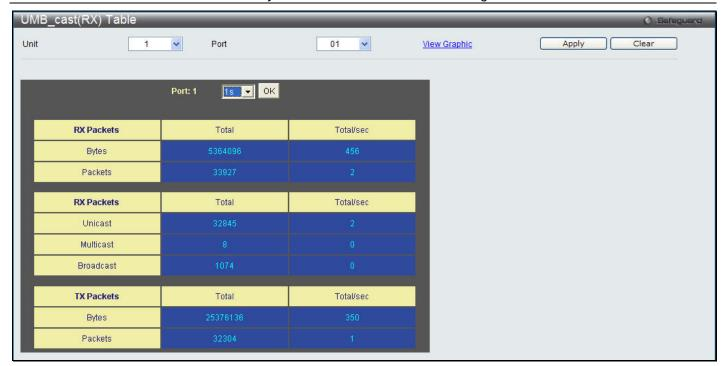
Figure 11-7 RX UMB\_cast (RX) Table window (table for Unicast, Multicast, and Broadcast Packets)
