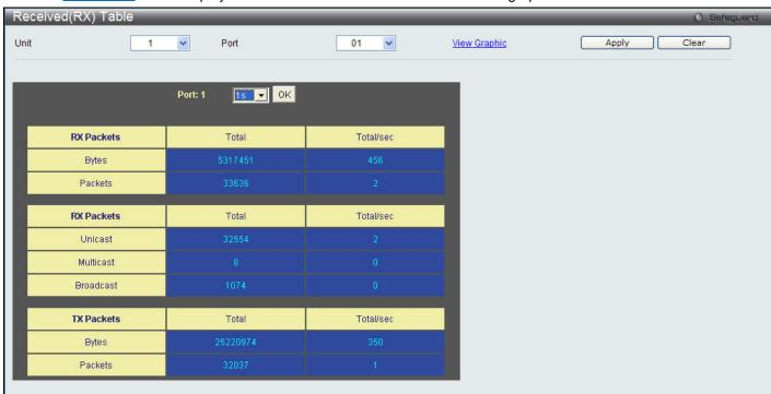
Figure 11-5 Received (RX) Table window (for Bytes and Packets)
