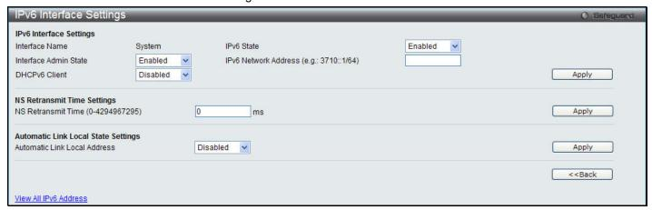
Figure 3-11 IPv6 Interface Settings – IPv6 Edit window
