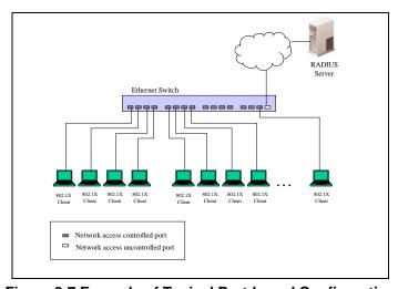
Figure 8-7 Example of Typical Port-based Configuration
