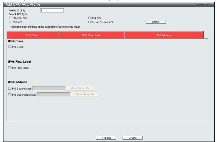
Figure 7-34 Add CPU ACL Profile (IPv6 ACL)
