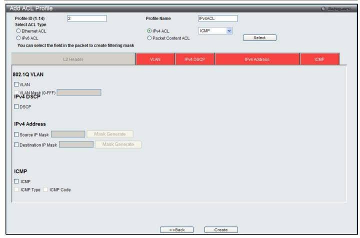
Figure 7-8 Add ACL Profile window (IPv4 ACL)
