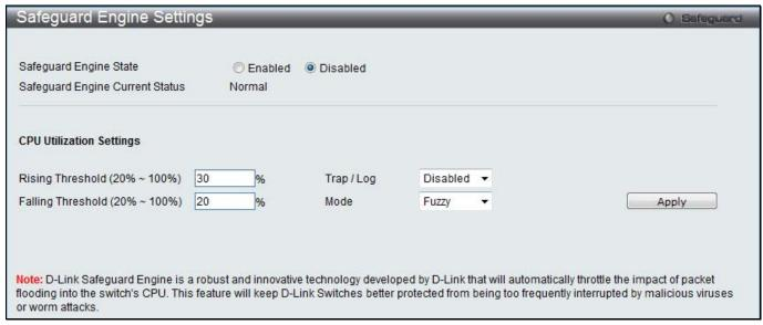
Figure 8-75 Safeguard Engine Settings window
