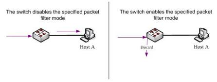
Figure 4-53 Method of dealing with the specified packet
