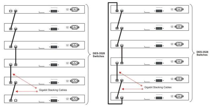
Figure 2-18 Switches stacked in a Duplex Chain
