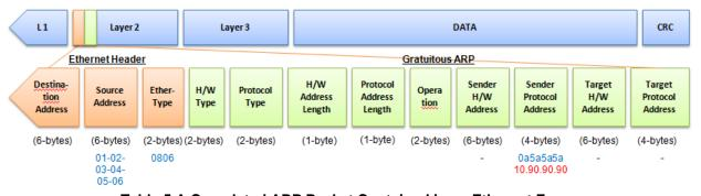
Table 5 A Completed ARP Packet Contained in an Ethernet Frame
