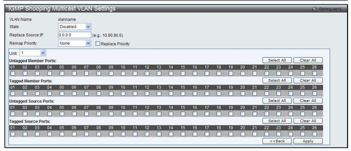
Figure 4-68 IGMP Snooping Multicast VLAN Settings - Edit window
