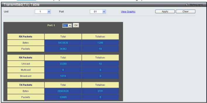
Figure 11-9 Transmitted (TX) Table window (table for Bytes and Packets)
