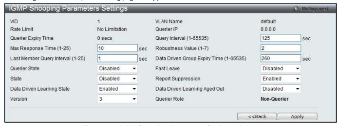
Figure 4-43 IGMP Snooping Parameters Settings window
