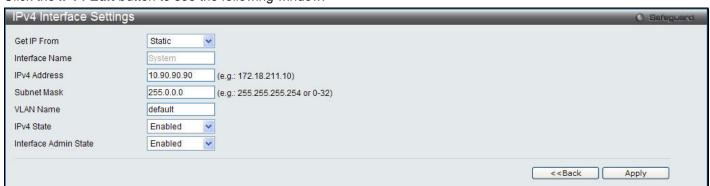
Figure 3-10 IPv4 Interface Settings – IPv4 Edit window
