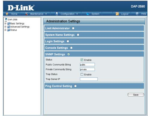
**Trap Server IP:** Enter the trap server IP address. This is the IP address of the SNMP manager to receive traps sent from the wireless access point.
