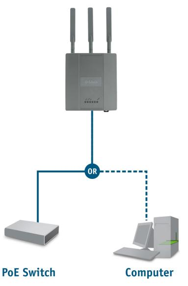
Connect one end of an Ethernet cable (included with your package) to the LAN port on the DAP-2590 and the other end of the Ethernet cable to either your computer or to your PoE switch. The AP can be powered on by a PoE switch or by the power adapter shipped with the AP.
