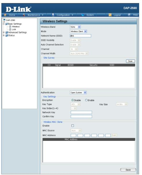
Authentication:Use the pull-down menu to choose Open System or WPA Personal.<br/>Select Open System to communicate the key across the network.<br/>Select WPA-Personal to secure your network using a password and dynamic key changes. No RADIUS server is<br/>required.For more information about the different types of Authentication offered on the DAP-2590 and the respective settings of<br/>each, please go to the first page of the Authentication explanations which begins on page 23.
