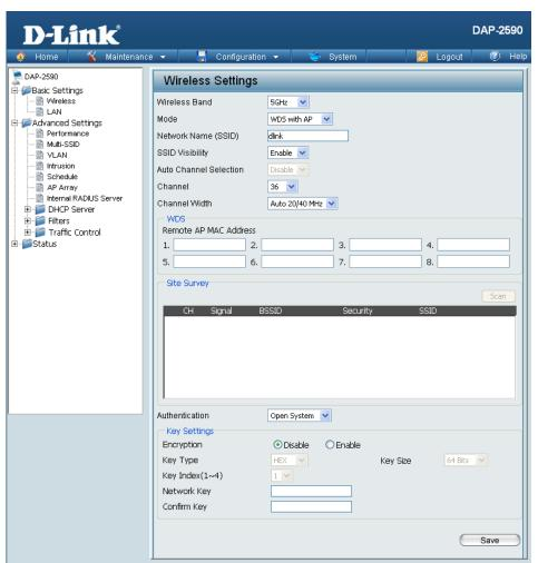
**Channel:** All devices on the network must share the same channel. To change the channel, use the pull-down menu to make the desired selection. (*Note: The wireless adapters will automatically scan and match the wireless settings.*)
