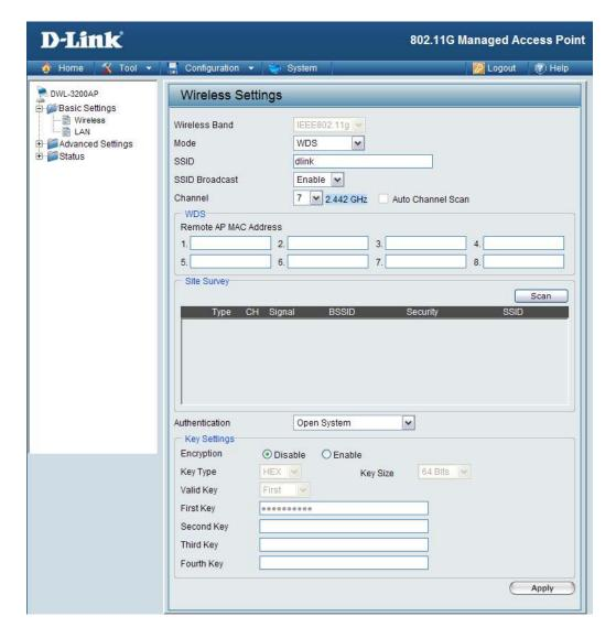
In WDS mode, the DWL-3200AP wirelessly connects multiple networks, without functioning as a wireless AP.
