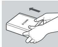
2. Slide the top cover away from you until it unhooks from the base (note the direction of the D-Link logo in the image to verify the direction).
