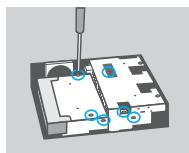
5. Use all six screws supplied to secure the hard drive to the base unit.
