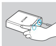
8. Re-attach the device screws at the bottom of the DNS-315.
