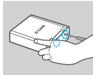
1. Use a screwdriver (not supplied in box) to unscrew the two screws at the bottom of the DNS-315.
