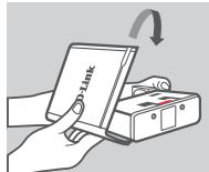
6. Flip the cover back to align with the red line on the bracket.
