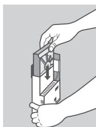
4. Keeping the DNS-315 in the upright position, insert a compatible 3.5" hard drive into the drive bay of the device. (Ensure the SATA connector is aligned with the SATA socket at the base of the unit otherwise the DNS-315 will not power on correctly).
