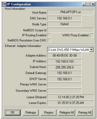
The important settings to watch for in this screen are in the **Host Information** box. Make sure that the DNS Servers box has the
