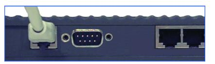
Using CAT5 UTP cable, connect each computer that is equipped with an Ethernet adapter to one of the **four Ethernet LAN** ports on the DI-704P.
