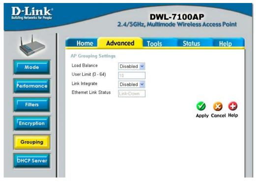
When you **Enable Load Balance** you allow several DWL-7100APs to balance wireless network traffic and wireless clients among the DWL-7100APs in the network. Assign each access point a different **non-overlapping channel** (e.g., 1, 6, 11).
