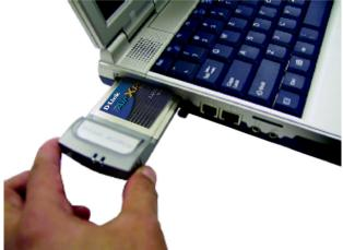
C. Gently insert the DWL-AG650 into the Cardbus slot in your laptop computer (as shown.)
