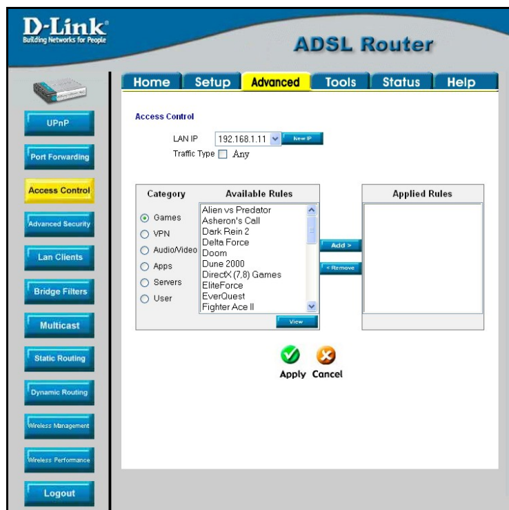
Figure 4-7. Access Control menu
