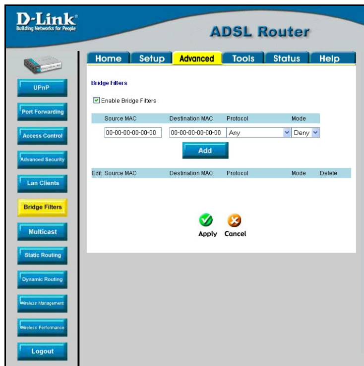
Figure 4-9. Bridge Filters menu
