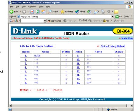
You can setup 16 LAN-LAN profiles, that is to say you can connect to 16 remote networks. Select an available index. Give an appropriate name for the profile, and enable it.
