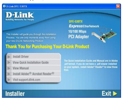
If you do not have auto-execute enabled for your PC's CD-ROM drive, navigate to the root directory of the CD using Windows Explorer and click on the file named **Autorun.exe**. This will open the window shown above. Then click the **Install Driver** link to install the driver.
