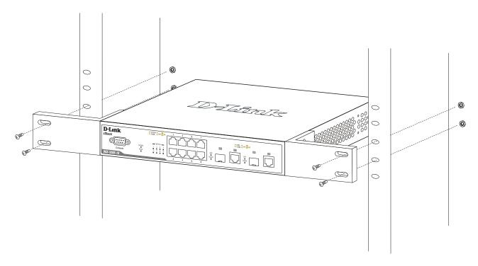
Figure 2- 5. Installing the DGS-3200-10 in a rack
