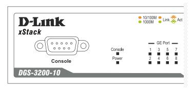
Figure 1-3. LED Indicators for DGS-3200-10
