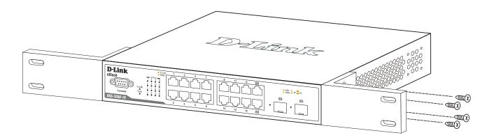
Figure 2- 4. Fasten mounting brackets on the DGS-3200-16
