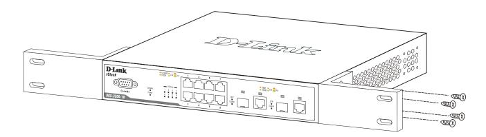
Figure 2- 3. Fasten mounting brackets on the DGS-3200-10
