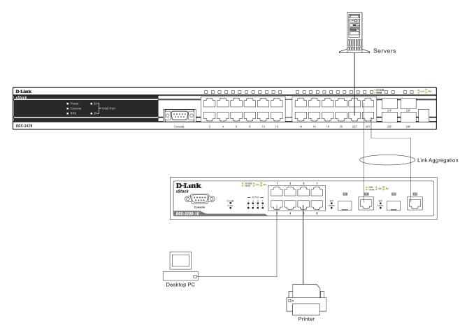
Figure 3-3. An example of a typical DGS-3200-10 connection
