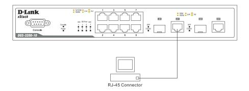
Figure 3- 5. Uplink connection to a server, PC, or switch stack
