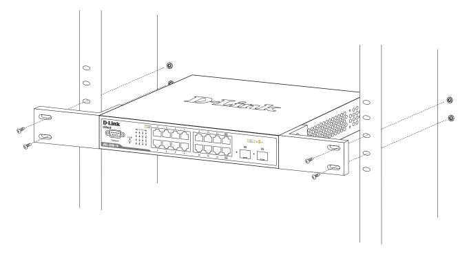
Figure 2- 6. Installing the DGS-3200-16 in a rack
