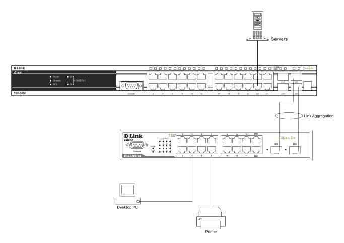
Figure 3- 4. An example of a typical DGS-3200-16 connection
