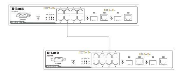
Figure 3- 1. Connect the DGS-3200-10 to a port on a switch with straight or crossover cable
