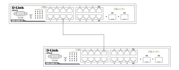
Figure 3- 2. Connect the DGS-3200-16 to a port on a switch with straight or crossover cable
