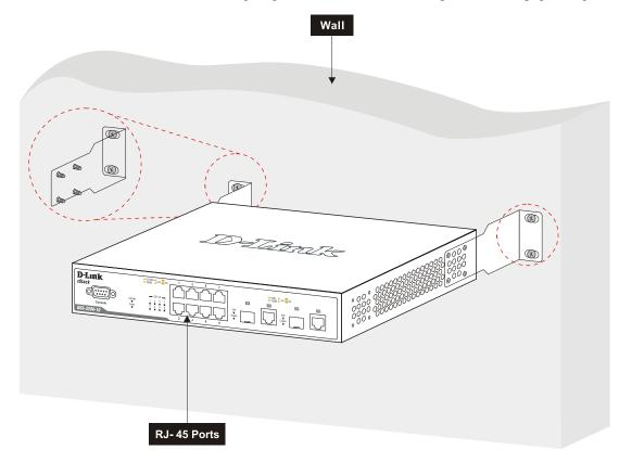
Figure 2-7. Fasten mounting brackets on the back of the DGS-3200-10 to a wall
