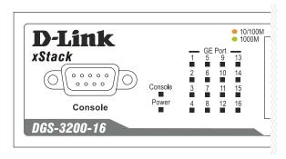
Figure 1-4. LED Indicators for DGS-3200-16
