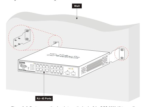
Figure 2-8. Fasten mounting brackets on the back of the DGS-3200-16 to a wall
