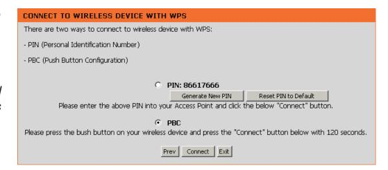
On the device you want to connect to, start the PBC process on the device. You will have 2 minutes to start the PBC process on both devices.
