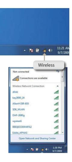
Highlight the wireless network (SSID) you would like to connect to and click the **Connect** button.
