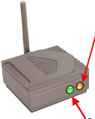
**Wireless Link/Act** – a steady **Orange** light indicates a good wireless connection. A blinking light indicates that the DWL-810 is receiving/transmitting from/to the wireless network.
