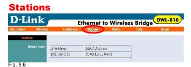
Click on **Stations** in the menu. A **Stations** table will appear, as shown here, providing information regarding the device connected to the DWL-810.
