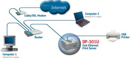
**Warning!** Only a USB printer may be connected to the USB port of the DP-301U. Do not connect any other USB device to the USB port; to do so may damage the unit, voiding the warranty for this product.
