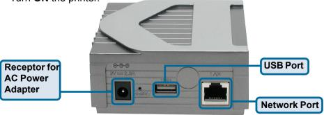
Then, plug one end of the power adapter into the DP-301U and the other end into your electric outlet. The DP-301U will turn on and begin a self-test.
