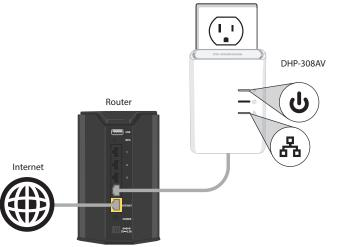
2 Plug in the DHP-W310AV Adapter in the room that you want additional wireless coverage and/or an Ethernet connection.
