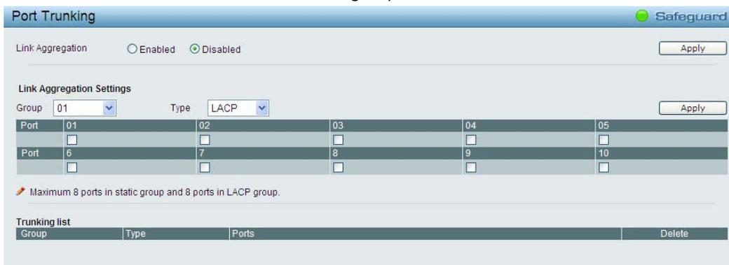
Figure 5.45 – L2 Functions > Link Aggregation > Port Trunking
