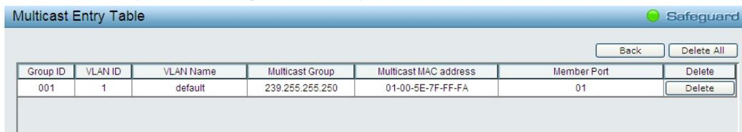
Figure 5.45 – L2 Functions > Multicast > IGMP Multicast Entry Table
