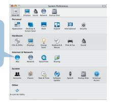
Select Built-in Ethernet in the show pull down menu Select Manually in the Configure pull down menu
